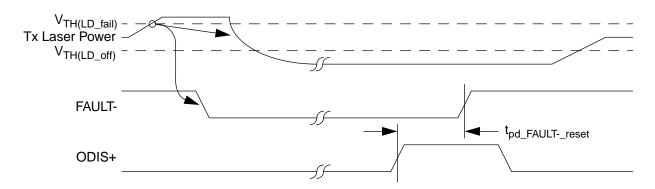
Figure 2: Module Fault interface timing Example
