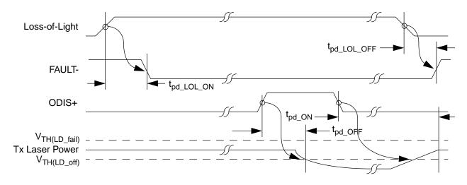
Figure 3: Typical Interface Operation for Link FAULT- Event
