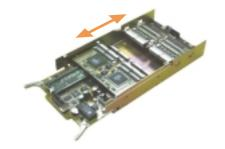
The controller itself is hot-swappable for full non-stop redundant operation. The backplane holding the cable connections is joined or separated from the main controller board by a docking connector. A faulty controller is easily removed and replaced.
