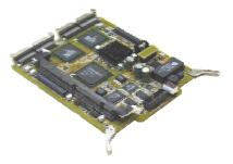
SentinelRAID controllers are ideal solutions for OEM customers who want to design their own backplanes. The controller board can fit the mechanical design of their backplane. This makes cableless, hot-swappable enclosures possible. Daughterboards with an M or FM suffix are designed for this application.
